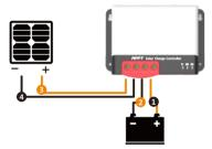
Awarning: Danger, Electric shock hazards! We strongly recommend connect a fuse or circuit breaker to the PV array and battery terminals to prevent electric shock hazards during wiring or error operation, and make sure that fuse or circuit breaker is disconnected before wiring.
