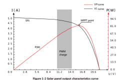
In addition, due to the difference in ambient temperature and light conditions, the maximum power point often changes. The MPPT controller can adjust parameters according to different conditions from time to time to keep the system near to its maximum working point. The whole process is fully automatic and does not require any adjustments by users.
